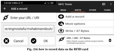
7- A message (Approach NFC Tag) appears, to bring the RFID card closer to the phone. If the writing process is done correctly, another message will appear stating that (write Complete) then the RFID card is ready and loaded with the link of the system, and it can be read from any RFID reader or any phone that has the feature (NFC).
