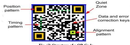
Fig. (3) Structure of a QR Code
