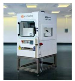
Fig (1) Nano-spider<sup>tm</sup> electro-spinning wire system
