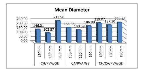
Fig (2) Effect of changing the spinning distance on the mean diameter values of nano-fibers
