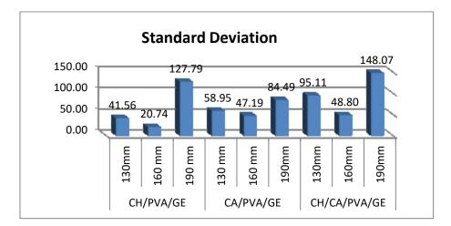
Fig (3) Effect of changing the spinning distance on the standard deviation values of nano-fibers
