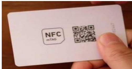
Fig. (18) Combine the Bar code, QR code with the RFID Card
