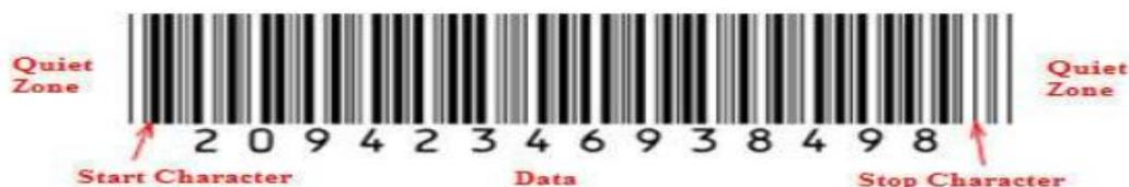
Fig. (1) Barcode structure
