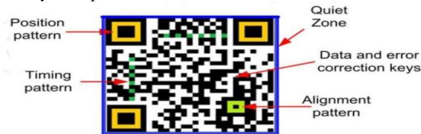
Fig. (3) Structure of a QR Code
